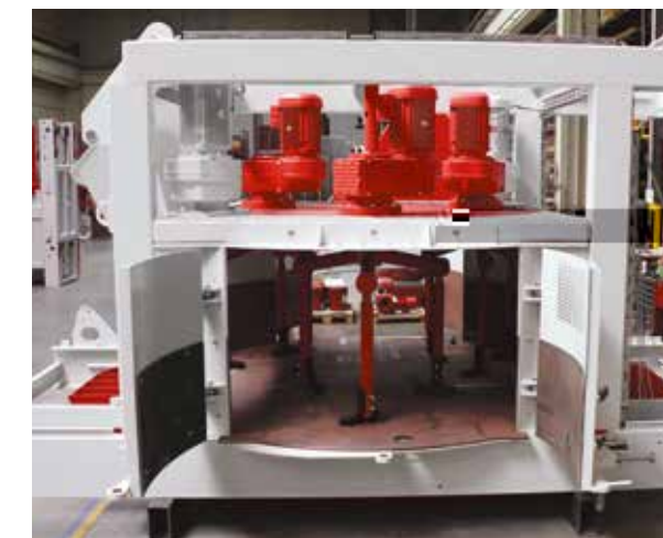
SM 3375 with double-sided access for cleaning and maintenance
