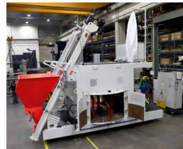
Mixer SM 2250 with large access for cleaning and maintenance
